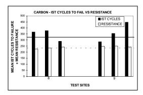
Both carbon test sites had at least 2 panels that met of exceeded the mean performance.
