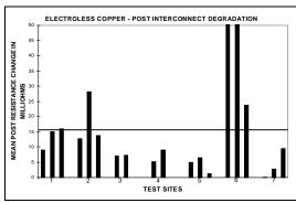
Two of the seven electroless copper test sites had at least 1 panel that exhibited post separation. All 3 panels in test site 6, clearly exhibited gross post separation.
