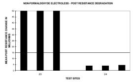
All 3 panels for non-formaldehyde electroless copper test site 23 clearly exhibited gross post separation.
