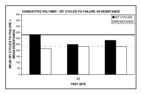
The single conductive polymer test site had one panel that met or exceeded the mean performance.
