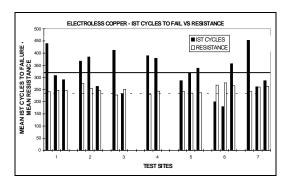
All electroless copper test sites had at least 1 panel that met or exceeded the mean performance. For the panels that did not achieve the mean performance, it can be seen that the mean resistance column was above the reference line (thinner copper). The exception was test site #6, which exhibited a high degree of post
