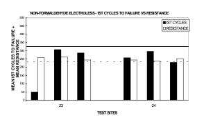
Neither non-formaldehyde electroless copper test site met or exceeded mean performance. Test site 23 exhibited a high degree of post separation (see post separation results section for an explanation of results).
