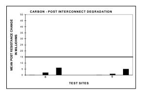
No post separation was detected on any carbon panels.
