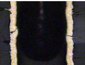
**Photo 5** – Microsection of a non-filled via from Lot 1 showing a classic fatigue failure at high CTF.
